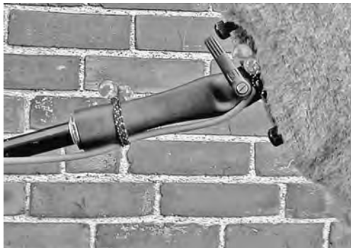
Figure 7.12 Hairballs in use. Not only do they keep things neat; they also let you know that this mic is pointing down.
